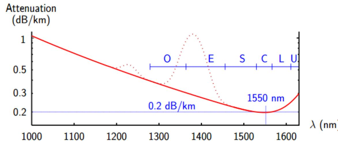
Can use optical amplifiers to avoid signal regenerators (O-E-O conversion)
