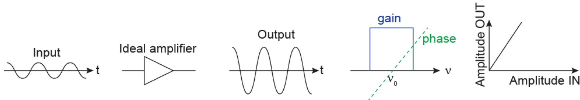
Linear system: amplitude of input signal increased by fixed factor
